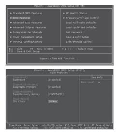
BIOS provides you a set of basic values for your processor selection instead of the jumper settings. The processor speed can be manually set from the <BIOS Features> menu screen.
