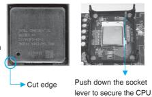
3. When the CPU is in place, press it firmly on the socket while you push down the socket lever to secure the CPU. The lever clicks on the side tab to indicate that it is locked.
