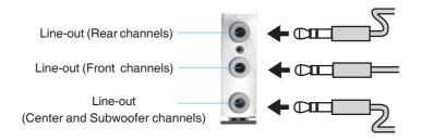
**Description:** Both Line-in and Microphone are converted to Line-out under the 6-channel configuration.
