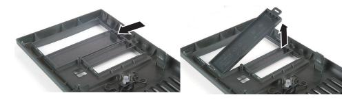
**5** Remove the shield for the bay into which you are installing the new drive.
