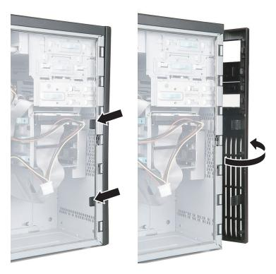
**4** Press the drive bay face plate release tab, then swing the faceplate away from the front cover and remove the face plate.
