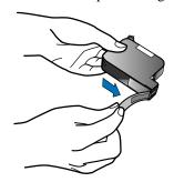
Push the black print cartridge firmly down into the slot on the right.
