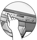
When your HP OfficeJet is on, a light appears on the front panel, and text appears in the front-panel display. If you do not see these, check the power cord connections from the back of the unit to the power-supply adapter and from the power-supply adapter to the power outlet.
