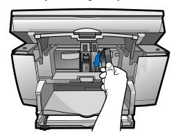
Lower each print-cartridge latch down onto the top of the cartridge, and push down until the latch locks firmly into place.
