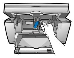
NOTE The print-cartridge label should be facing you after the cartridge is inserted.
