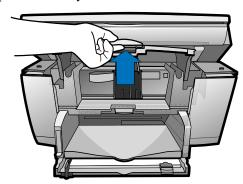
3 Remove the cardboard insert from the inside of the unit.
