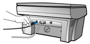
Plug the adapter end of the main power cord into the power supply adapter.
