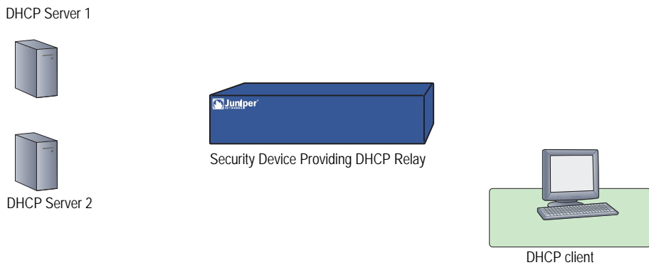
Figure 77: DHCP Relay Services Within a Vsys
